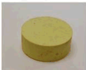
50 wt% AgI/50 wt% Glass 500°C for 3 hr
