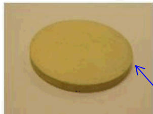
50 wt% AgI/50 wt% Glass, 500°C for 3 hr
