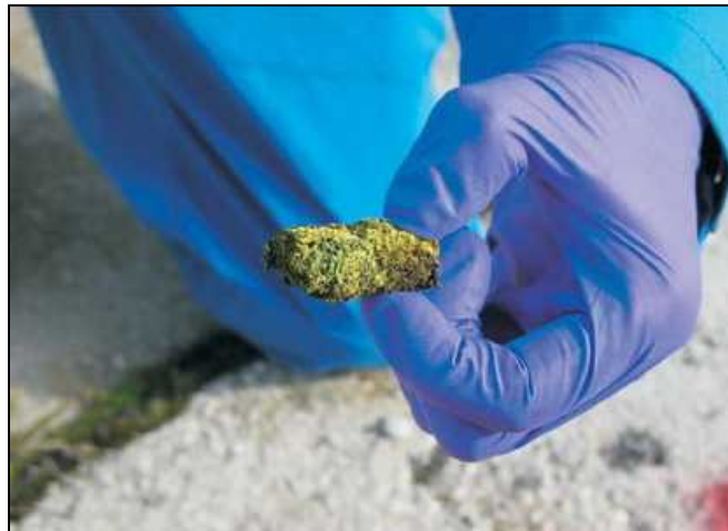
DU fragments fully corrode 25 - 35 years after impact
