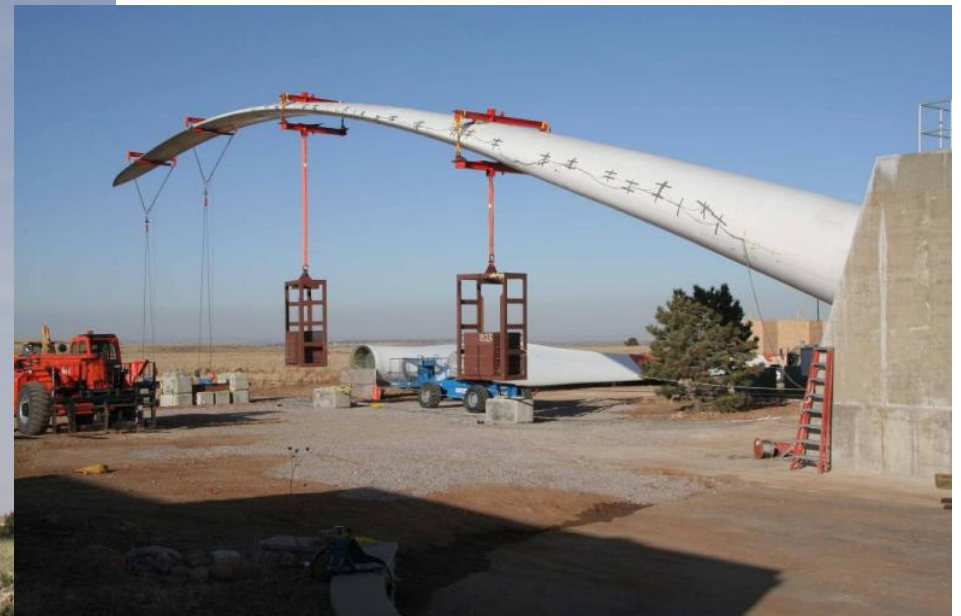
45 m blade test NREL/NWTC, CO
