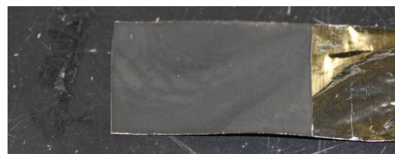
DW LiFePO 4 on copper current collector
