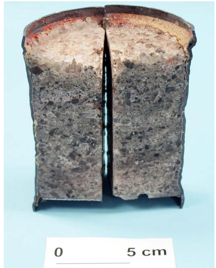
Figure 3. Post experiment crushed salt specimen compacted at 250°C.
