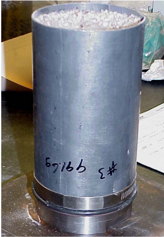
Figure 1. Crushed salt in lead jacket before compaction [3].
