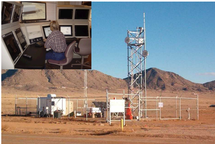
Sensor, camera, and communications array at the SNL Border Security System Test Facility
