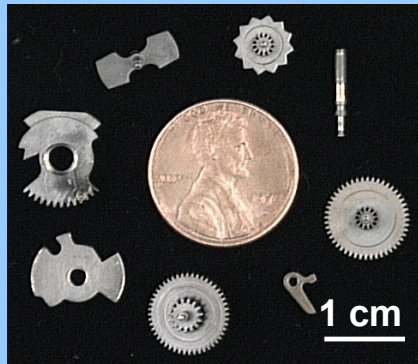
MoS 2 -lubricated machine parts
