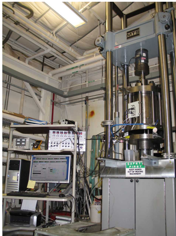
Figure 2. Testing system used to conduct quasi-static triaxial compression tests.
