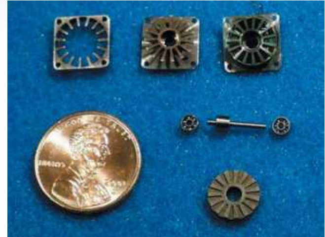
Meso-scale stepper motor machined by \mu WEDM process. Stepper motor size is 10 mm x 10 mm x 5 mm.
