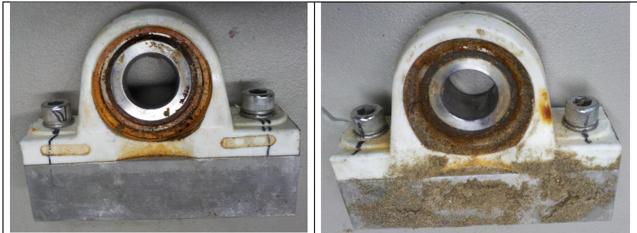
Figure 35: Seized Ball Bearings from Beta 1B River Installation
