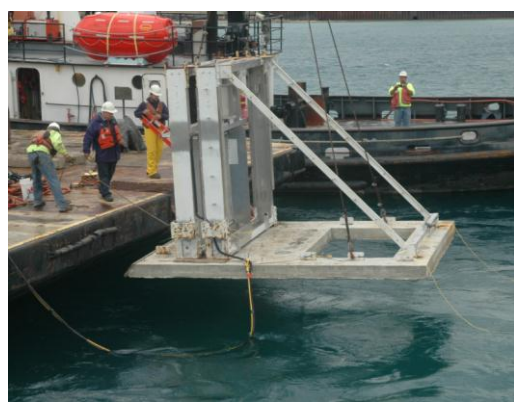
Figure 28: VIVACE Beta 1B Prototype Being Lowered in Water By Crane From Barge
