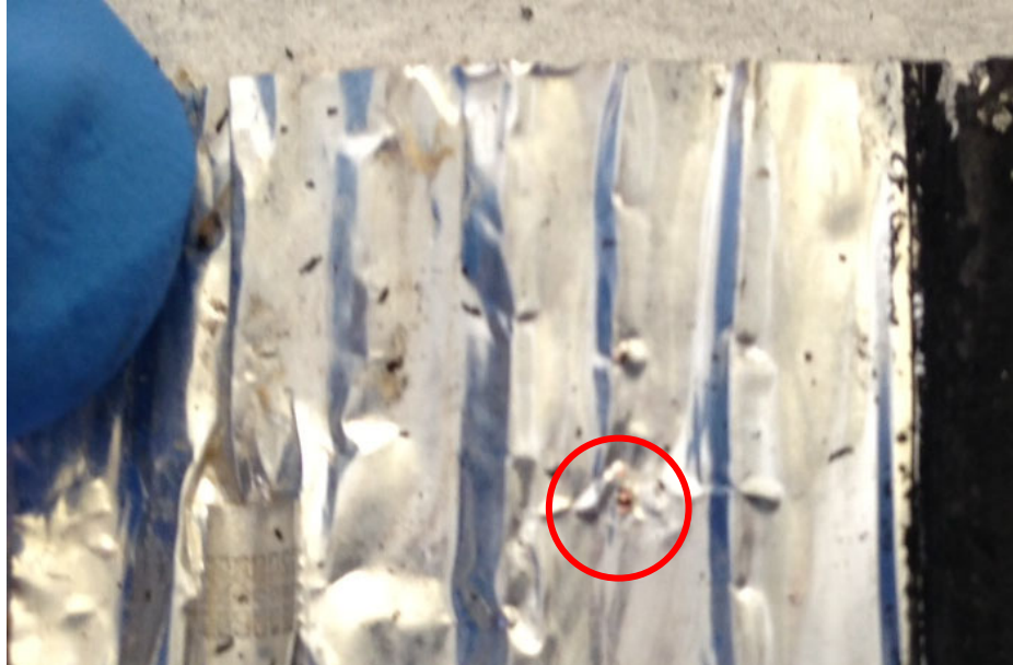
Figure 17: Photograph of a part of the cathode from Figure 16 showing a portion of bare aluminum foil that is a part of the core of the cell. The portion of the Al foil circled in red shows a hole in the aluminum foil and the underlying copper foil (from the anode coating) is clearly visible and likely responsible for an internal short circuit induced by melting of the separator between the anode and cathode layers.
