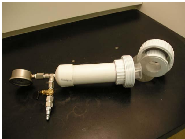
Photo 3. Unassembled BGST Showing Playtex Drop-In and SS Screen Position.
