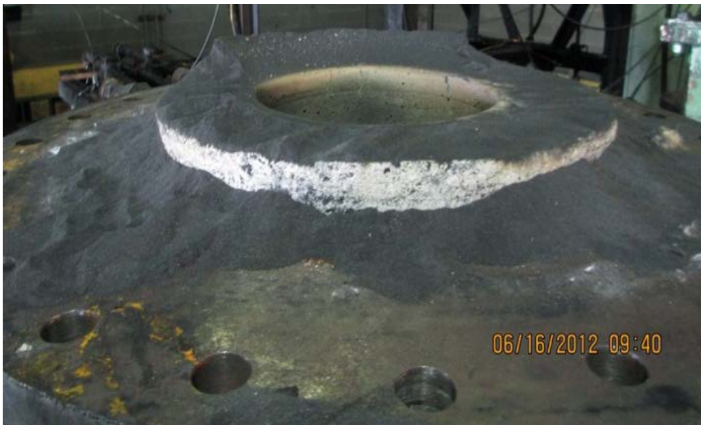
(a) Gap between the chamber 1 and 2, decent amount of carbon material was filling the gas
