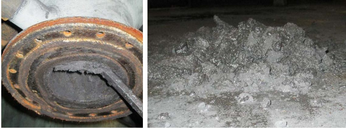
Fig 8. Carbon solids in the bottom cone of the afterburner
