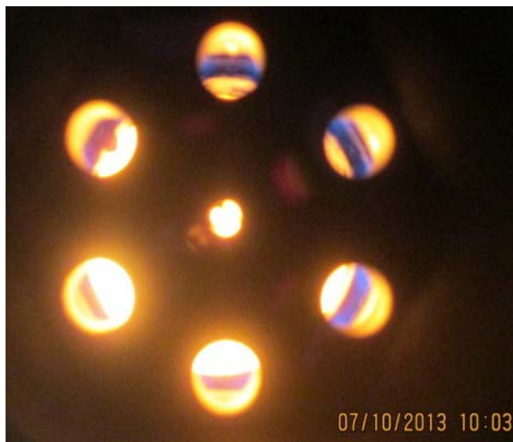
Fig 5. Flame in combustion chamber with 22 lbs/hr green coke feeding
