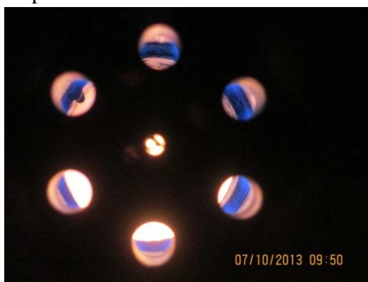
Fig 4. Pilot flame (no volatile, no extra compressed air)
