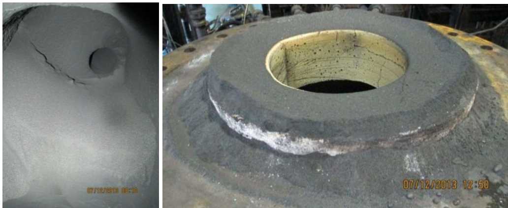
Fig 13. Carbon solids settled inside afterburner, in tee section (left) and between combustion chambers (right).
