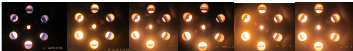
Fig 9. Combustion flame changes with increasing throughput (0→22→35→55→75→100 lbs/hr)
