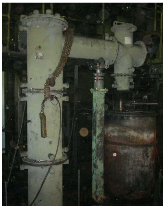
Figure 8. Afterburner configuration (a) and the top sections of installed system (b)
