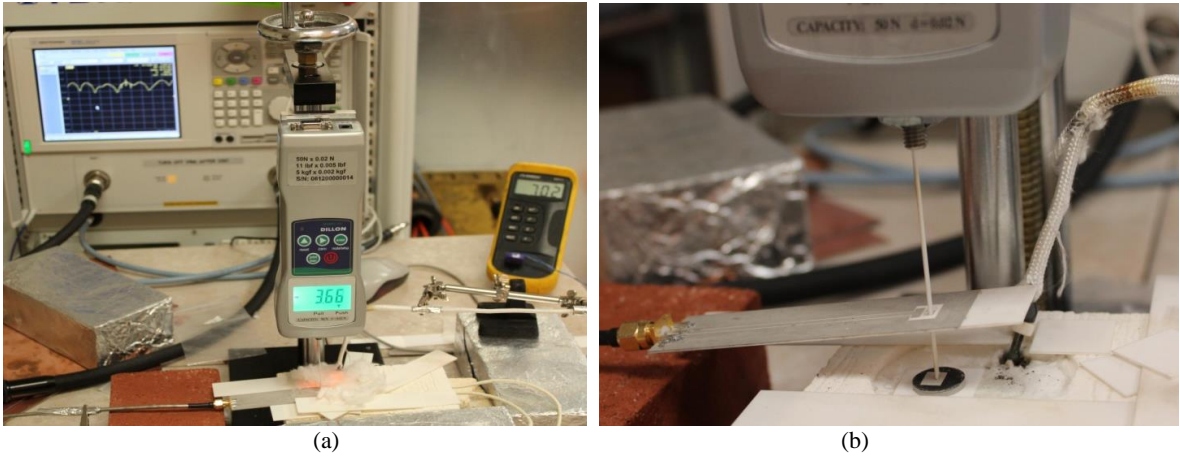
Fig. 32. (a) Pressure sensor measurement setup. (b) Exploded view of the interrogator antenna and the sensor on the heat pad.
