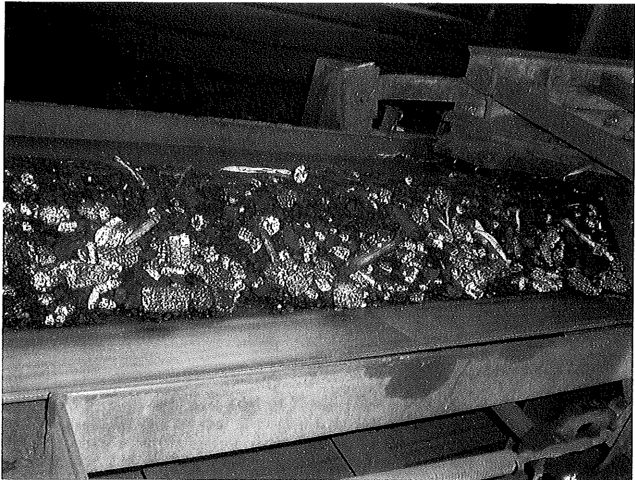
Bunker Fill Conveyor-PRB Coal & Chopped Corn Cobs
