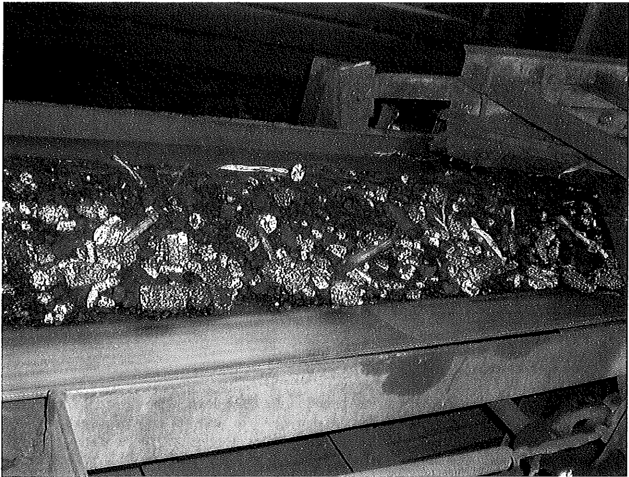
Bunker Fill Conveyor-PRB Coal & Chopped Corn Cobs
