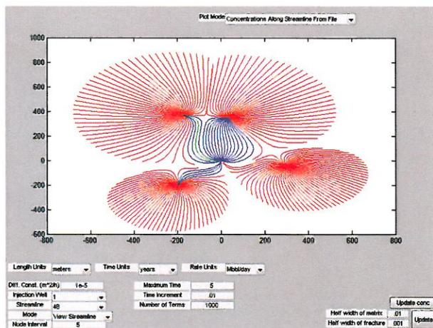
Figure 11: Streamline configuration: streamlines that don't reach a production well are shown in red, while streamlines that do are shown in blue and the streamline that concentrations were calculated for is shown in green
