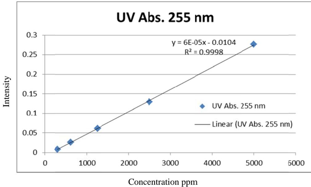
Figure 19. The peak UV absorption at 255nm is a linear function of TFT concentration.
