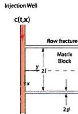
Figure 1: Assumed Geometry of Subsurface. Flow (in the  $y$ -direction) occurs from a source (red vertical bar) along fractures of width  $2d$  separated a distance  $2l$  apart.
