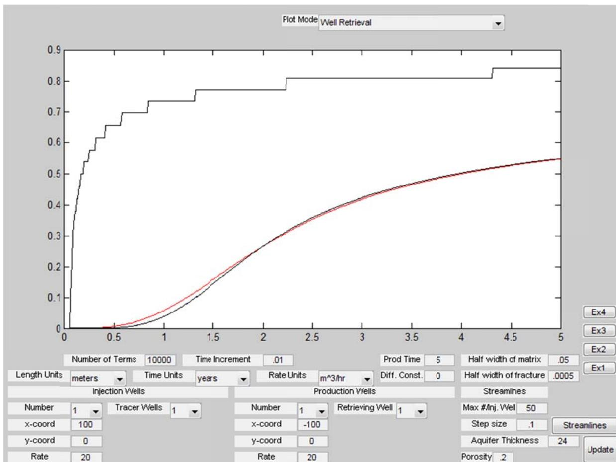
Tracer arrival curves for nanoparticles and TFT in supercritical CO<sub>2</sub> injected and produced at 20m<sup>3</sup>/m/day (equivalently 20 m<sup>3</sup>/hr over 24 m interval) from wells separated by 200 m. The diffusion constants for the tracers are as indicated in Table 2, the tortuosity of the pores in the matrix is 3, the fracture spacing is 10 cm, and the matrix porosity is 10%.
