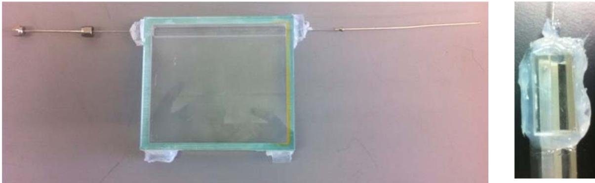
Figure 14. Glass apparatus encased in PDMS. Vacuum grease is applied at each connection to prevent any potential evaporation.
