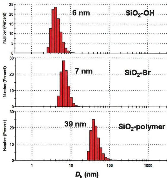
Figure C2. Size distribution of SiO<sub>2</sub> nanoparticle before and after polymerization.
