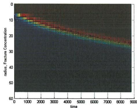
Figure 2: Fracture concentration for all time and position nodes. Diffusion constant of 2.8 cm<sup>2</sup>/s
