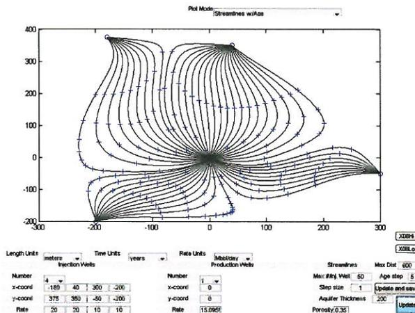
Figure 8: Simulated flow with a realistic well configuration and rates.
