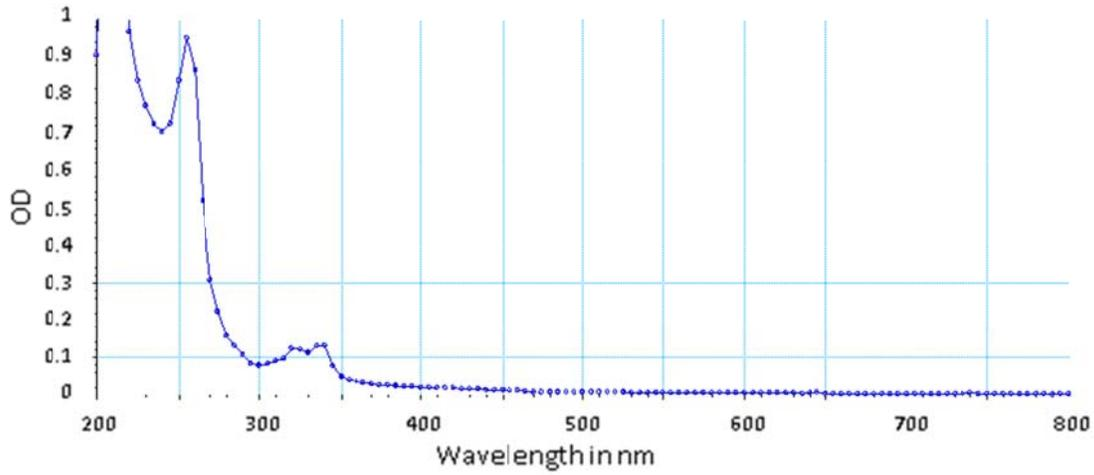
Figure 21. UV absorption profile for the chemical tracer TFT only (no silica nanoparticles).
