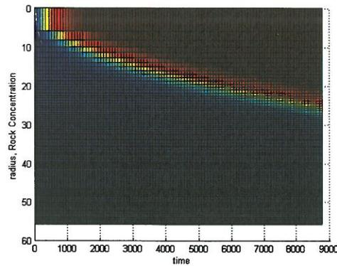
Figure 1: Rock matrix concentration for all time and position nodes. Diffusion constant of 2.8 cm<sup>2</sup>/s
