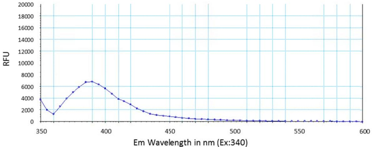
Solution and tracers are excited at 340 nm. The TFT is not fluorescent. The peak emission is at 390 nm. X axis is the wavelength in nm, Y axis is the intensity level.
