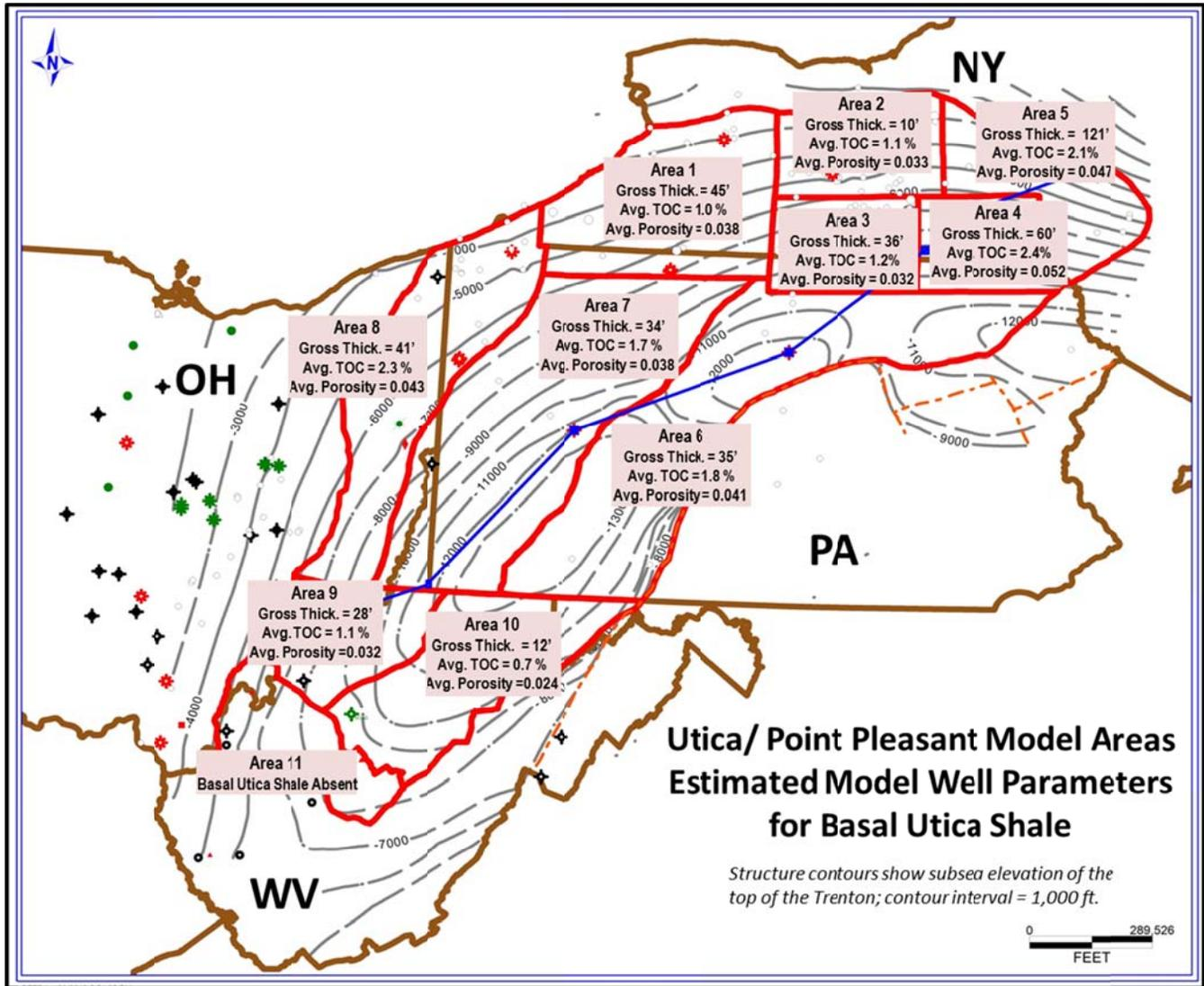
Figure 16. Upper (Shaley) Point Pleasant Reservoir Layer; Selected Model Well Parameters – Thickness, Average TOC, Average Total Porosity
