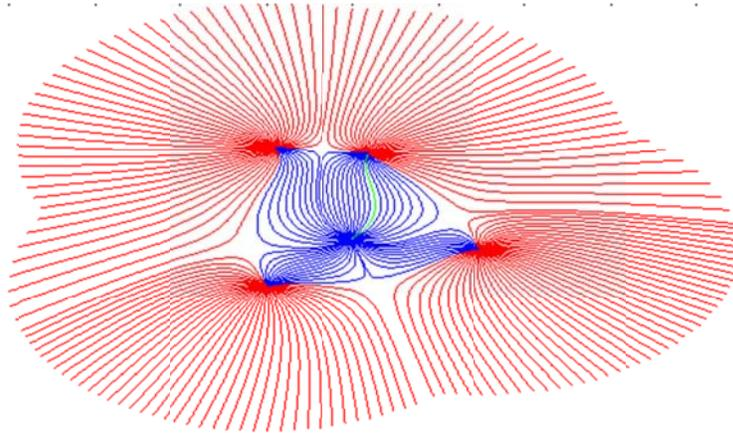
The red lines are streamlines emanating from the injection wells that do not connect to the production well; the blue streamlines are those that do connect to the production well. The streamlines were generated with the Gao matlab program developed for this project which is described in detail on Appendix B.
