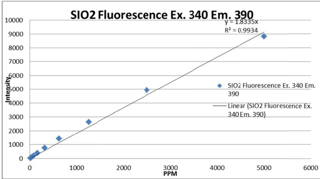
The relationship between the emission intensity (excited at 340 nm and measured at 390 nm) and the nanoparticle concentration is linear. The concentration of silica nanoparticles in Figure 18 is ~3700 ppm SiO<sub>2</sub> according to this calibration curve.
