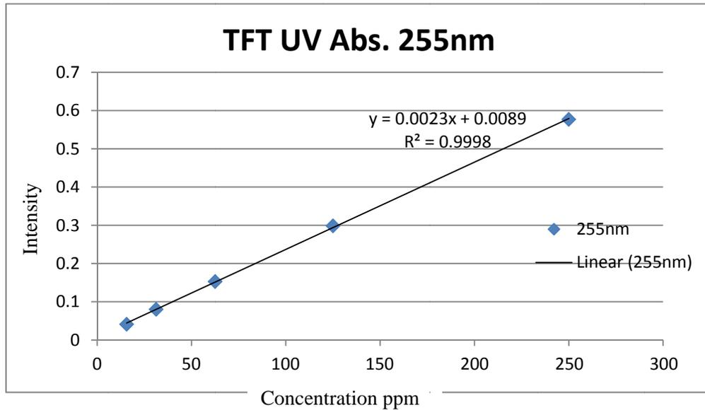
Figure 20 shows the UV absorption for SiO<sub>2</sub> nanoparticles and TFT, Figure 21 shows the UV absorption with the SiO<sub>2</sub> UV absorption subtracted out. The benzene peak height of ~2.6 in this figure indicates, via the calibration curve in Figure 19, that the TFT concentration of a little over 100 ppm.
