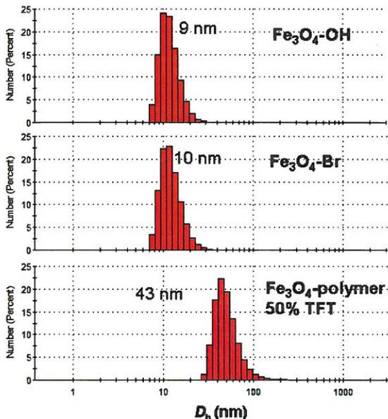
Figure C3. Size distribution for the Fe<sub>3</sub>O<sub>4</sub> nanoparticle before and after polymerization.
