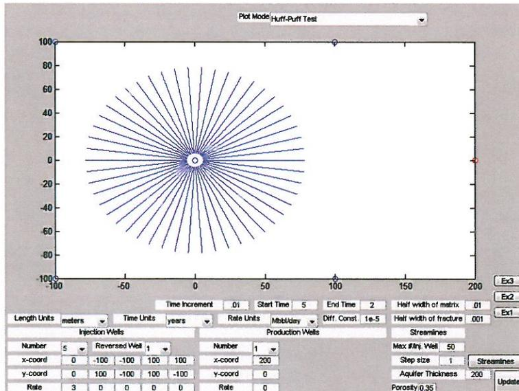
Figure 12: Well configuration for huff and puff test.
