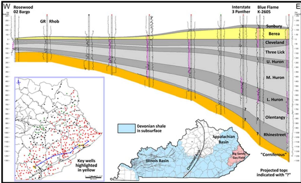
Uses the top of the Cleveland shale member of the Ohio shale, showing key wells. Dots on inset with location of cross section indicate wells for which digital wire-line log data are available for the shale interval
