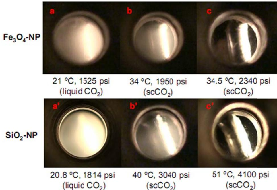
Fluid clarity (where you can clearly see the dividing bar of the cell) indicates the uniform dispersion of small nanoparticles. Cloudiness indicates the particles have clumped together to form clusters large enough to occlude light. The images indicate the nanoparticles are not dispersible in liquid CO<sub>2</sub> (not surprising as discussed in the text) but disperse well in supercritical CO<sub>2</sub>.
