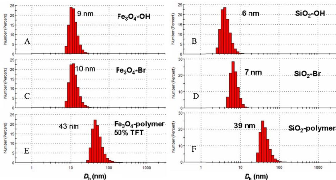
(A) bare Fe<sub>3</sub>O<sub>4</sub> particle; (B) bare SiO<sub>2</sub> particle; (C) Fe<sub>3</sub>O<sub>4</sub> nanoparticle with attached initiator; (D) SiO<sub>2</sub> nanoparticle with attached initiator; (E) Fe<sub>3</sub>O<sub>4</sub> nanoparticle after polymerization; (F) SiO<sub>2</sub> nanoparticle after polymerization.
