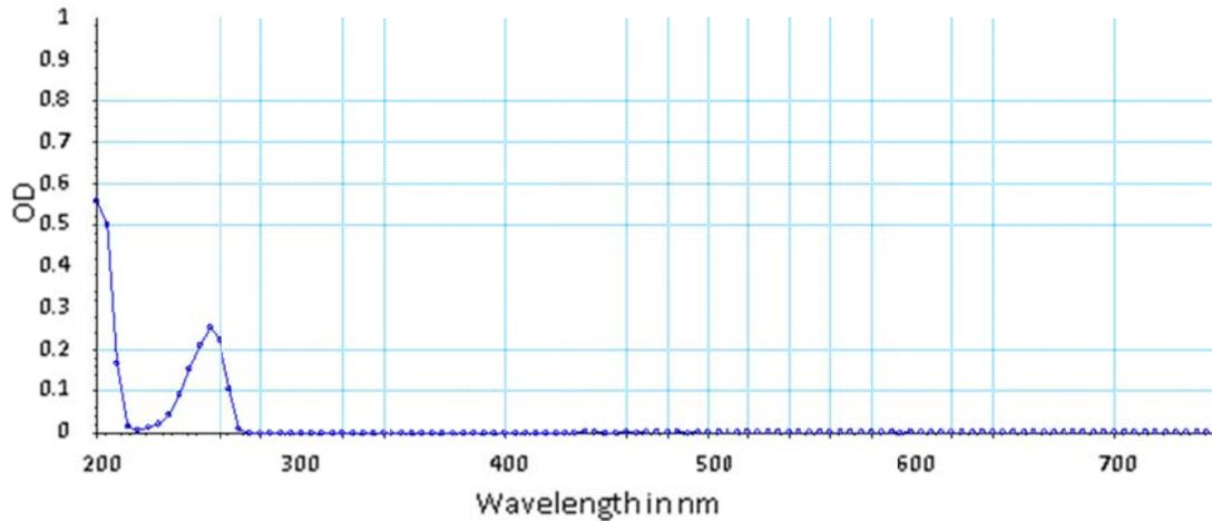
The UV absorption peak of benzene ring is at 255nm. There is no UV absorption after 280nm.
