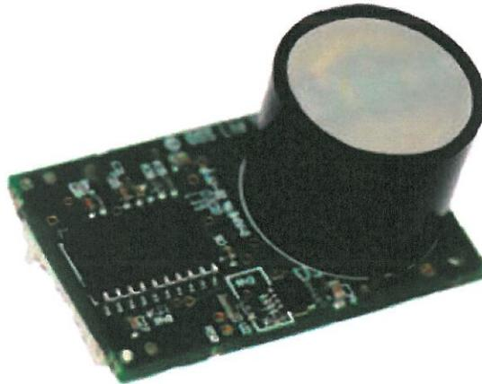
Fig. A2 – C20 CO<sub>2</sub> Sensor
