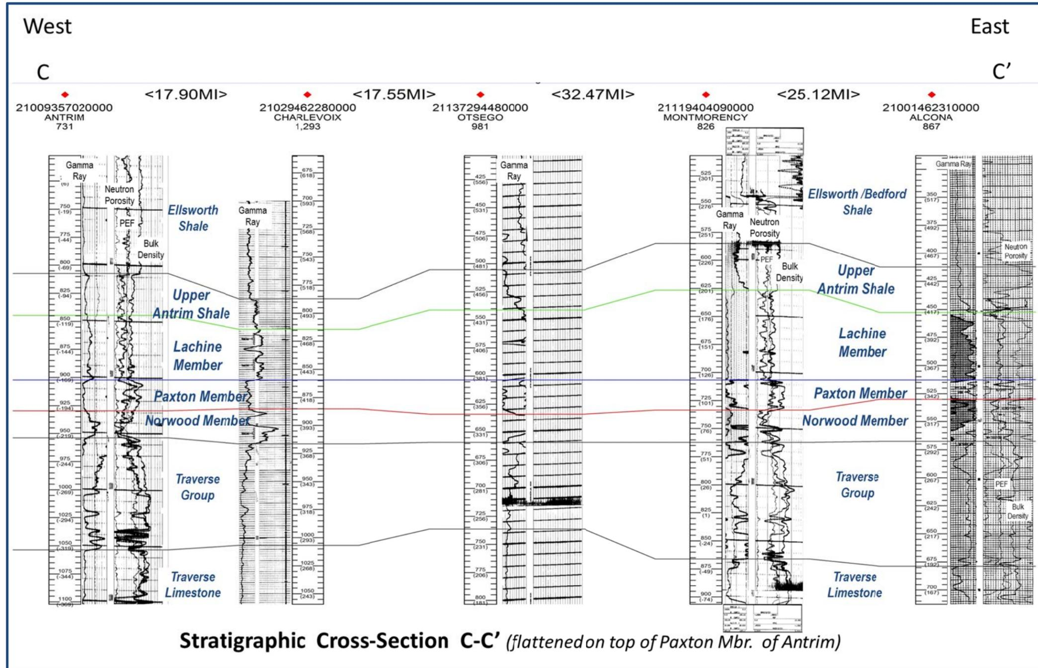
Figure 7: Antrim Shale Cross-Section C-C'
