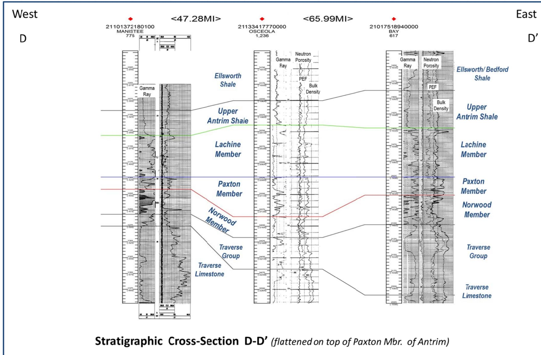
Figure 8: Antrim Shale Cross-Section D-D'
