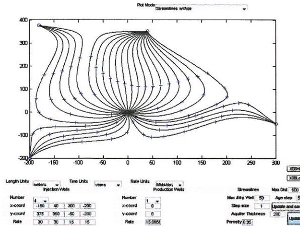
Figure 9: Simulated flow with same well configuration but higher injection rates
