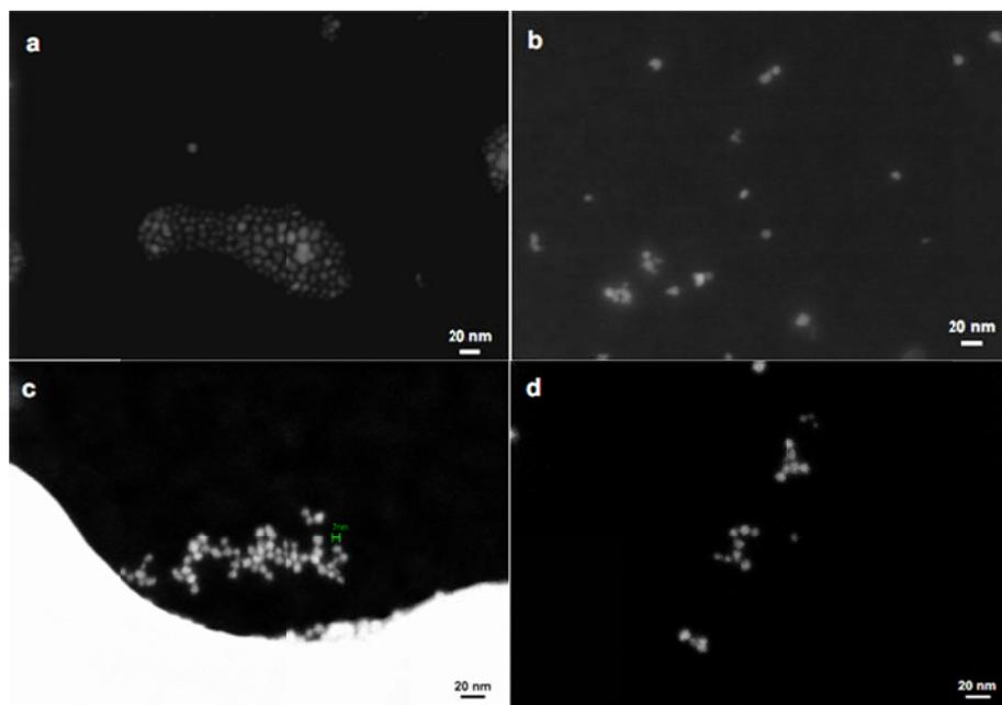
(a) shows the bare Fe<sub>3</sub>O<sub>4</sub> NP, (b) the polymerized Fe<sub>3</sub>O<sub>4</sub> NP, (c) the bare SiO<sub>2</sub> NP, and (d) the polymerized SiO<sub>2</sub> NP. Separation of the polymerized particles by their corona is evident in (b) and (d).
