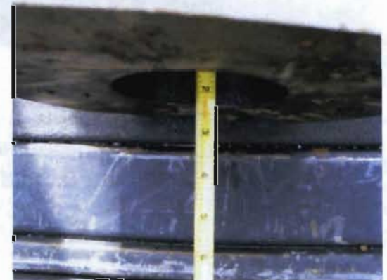
Piston depth measurement
