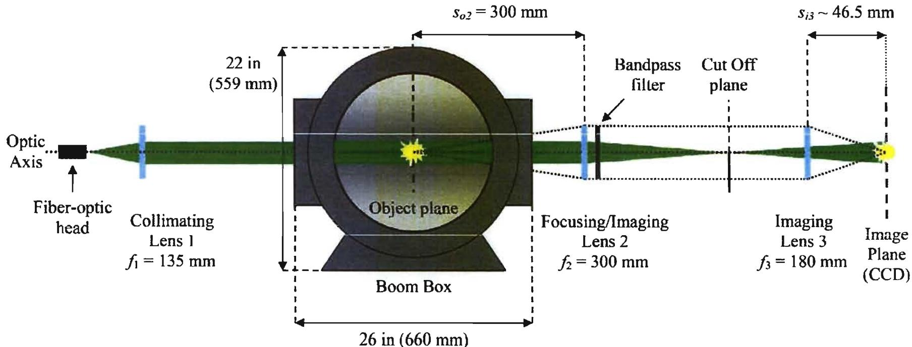
A cut-off mechanism can be utilized to directly visualize density gradients (schlieren imaging) or removed to directly visualize light deflection due to the density gradients (backlight imaging).
