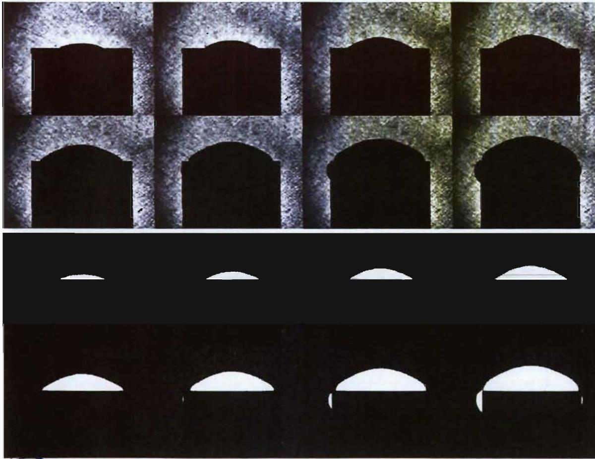
Image sequence depicts explosive breakout across the surface of the detonator by capturing the shock wave explosively-driven into PMMA.
