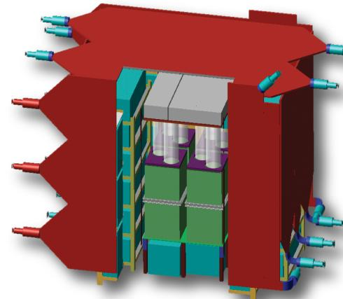
SONGS1: 0.64 tons of Gadolinium-doped liquid scintillator, monitored fuel composition through inverse  $\beta$ -decay
