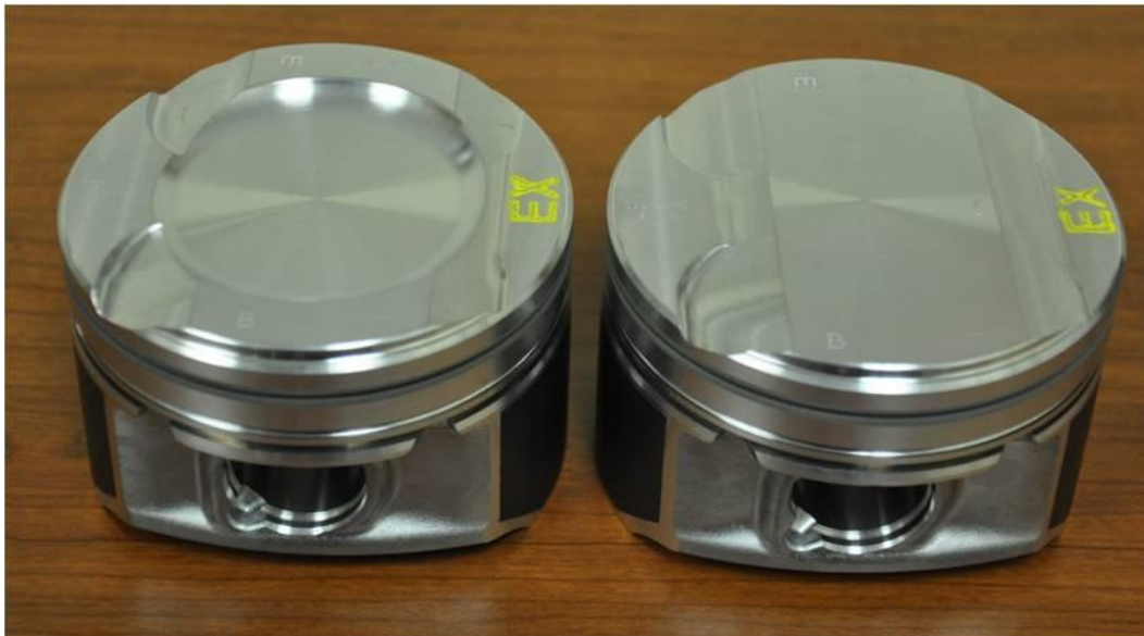
Figure 93: Modified engine piston with compression ratio of 12.5 and blank piston
