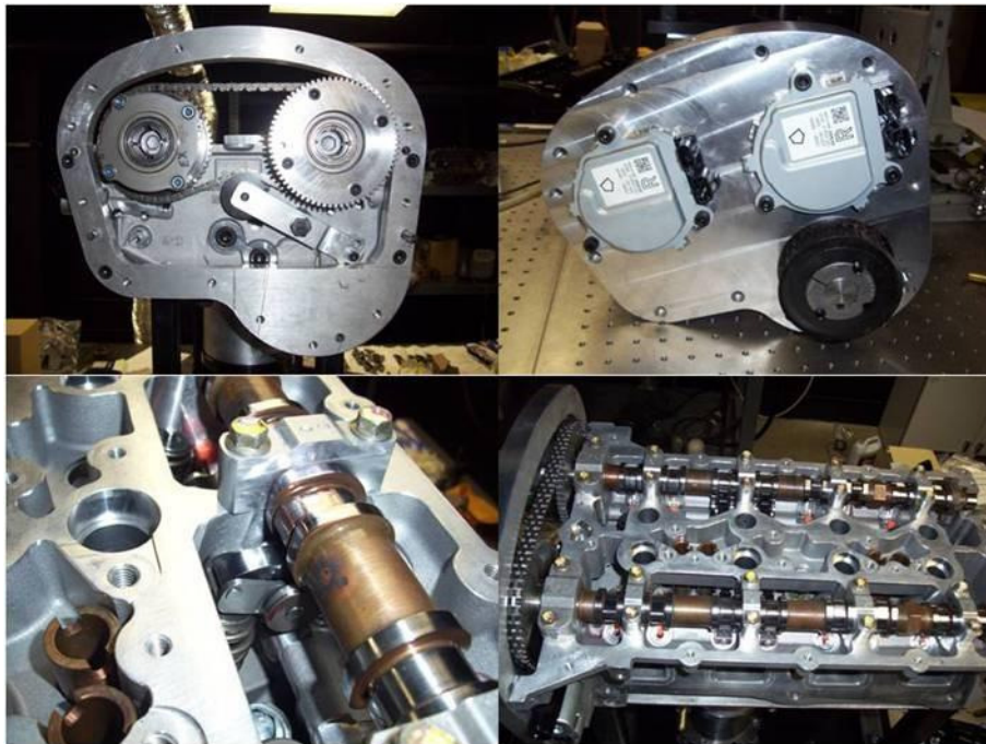
Figure 38: Cam phasing system and cylinder head with two step valve system
