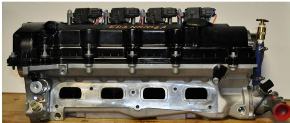
Figure 1: Target engine head provided by Chrysler for optical engine construction
