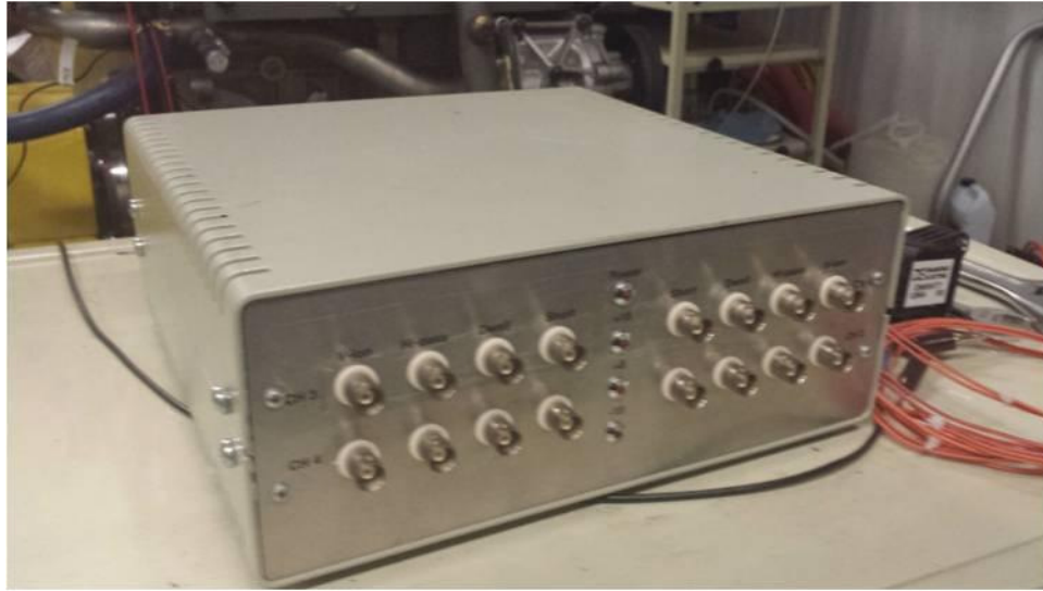
Figure 87: Prototype ionization capable ignition drive box
