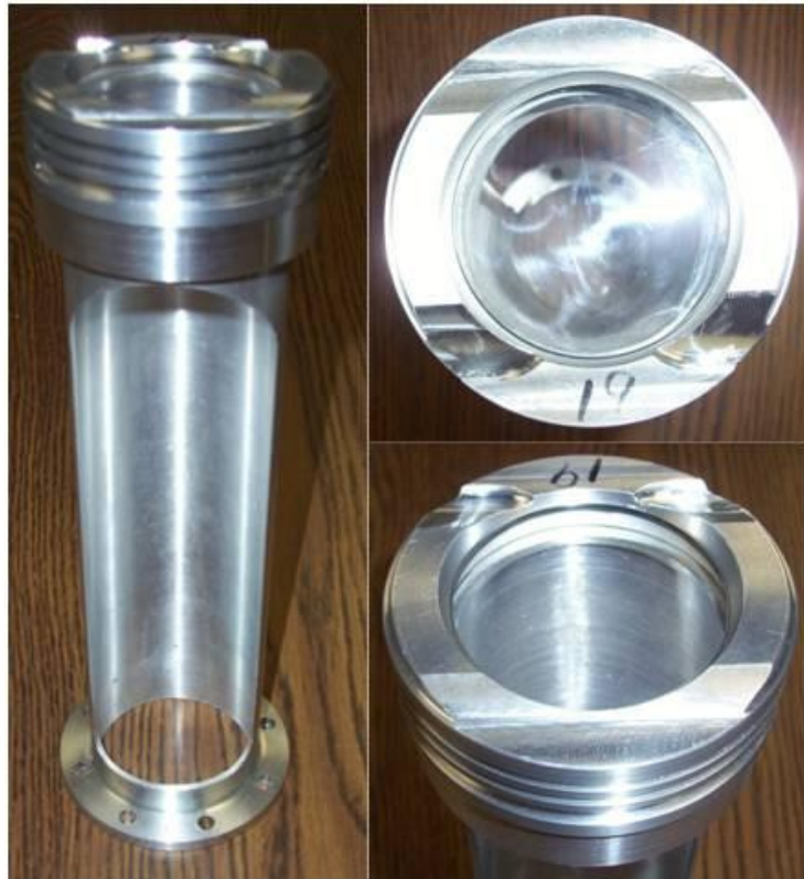
Figure 33: Constructed optical engine piston with optical lens
