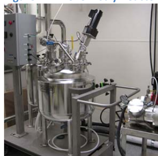
Figure A.12: Chemistry Reactor Skid (Pope)
