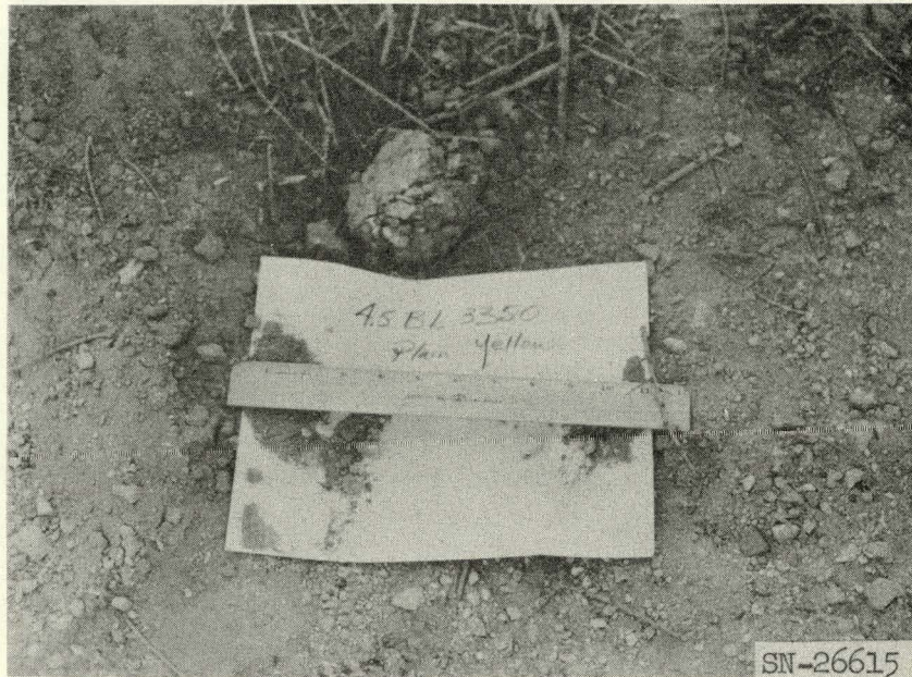
Fig. 4.5. Wall missile, recovered at 3350 feet, to left of collection strip; originally at 42 feet.
