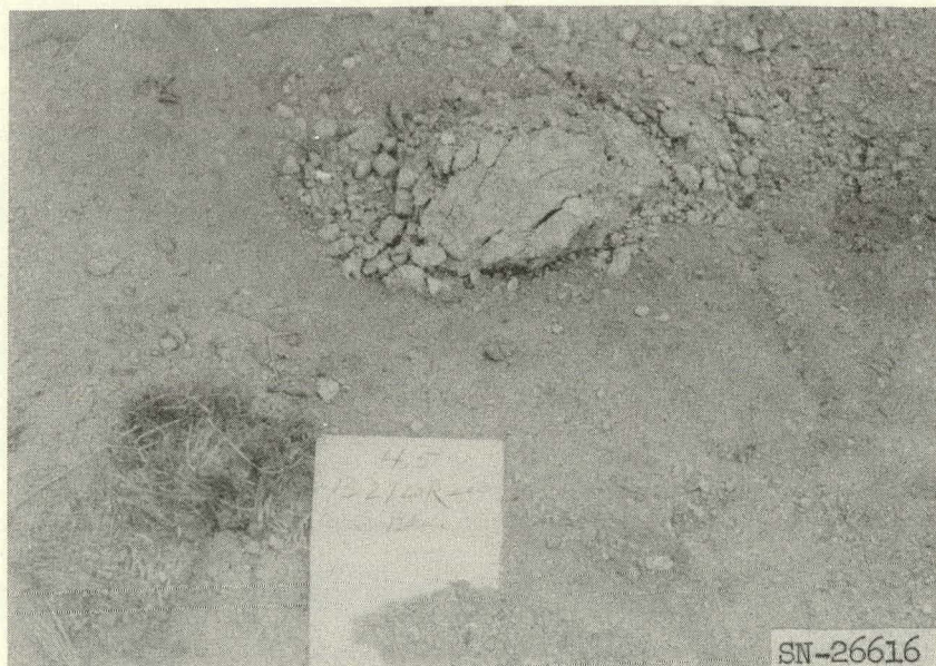
Fig. 4.6. Wall missile, recovered at 2720 feet, 200 feet to right of collection strip; originally at 50 feet. Note friability.
