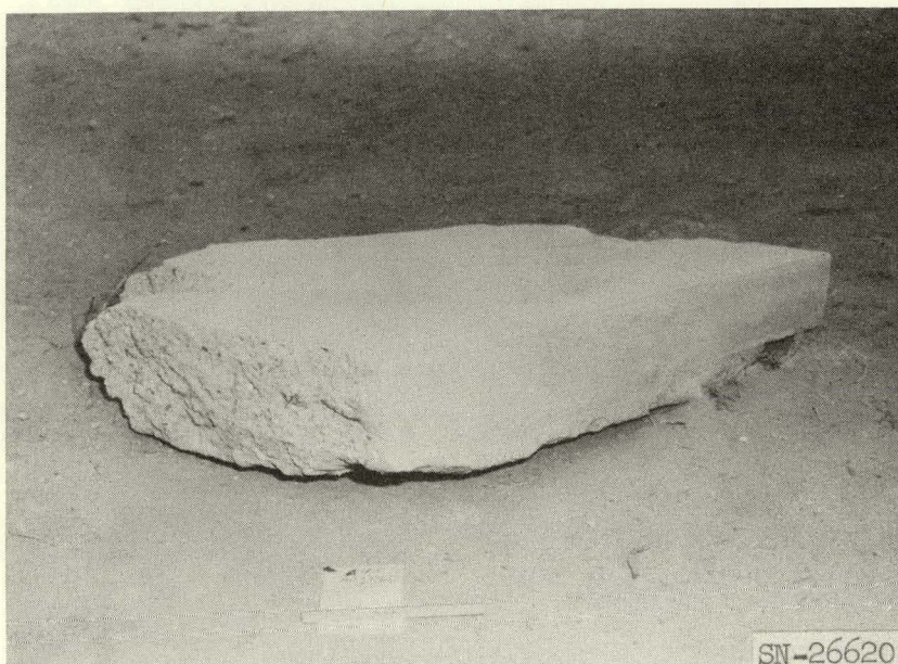
Fig. 4.11. Highway missile, found at 1000 feet, about 100 feet to left of center line; originally at 80 feet.
