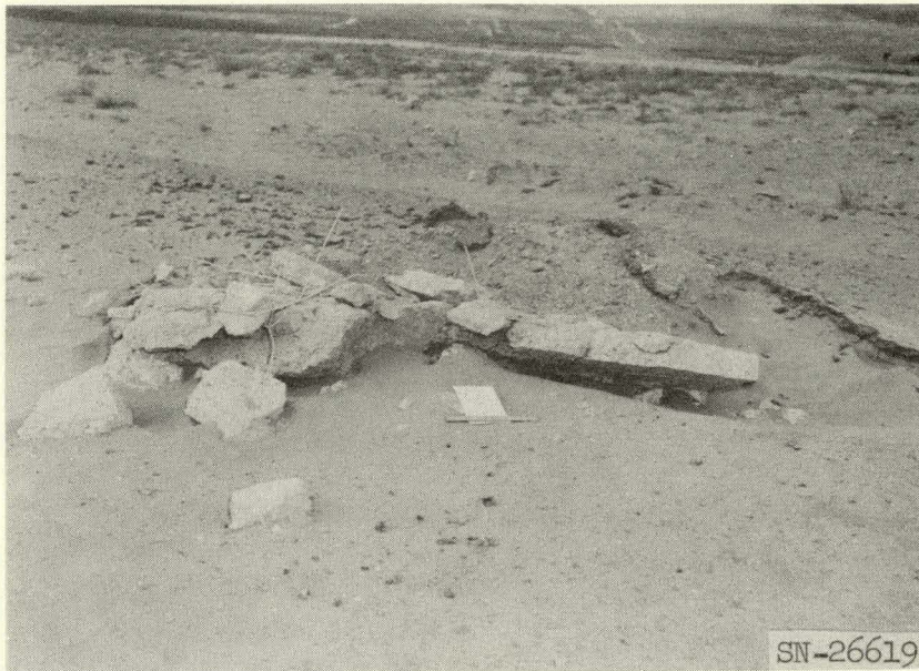
Fig. 4.10. Highway missile, found at 800 feet; originally at 80 feet.
