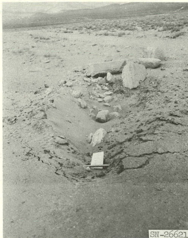
Fig. 4.12. Highway missile, found at 1200 feet; originally at 80 feet.
