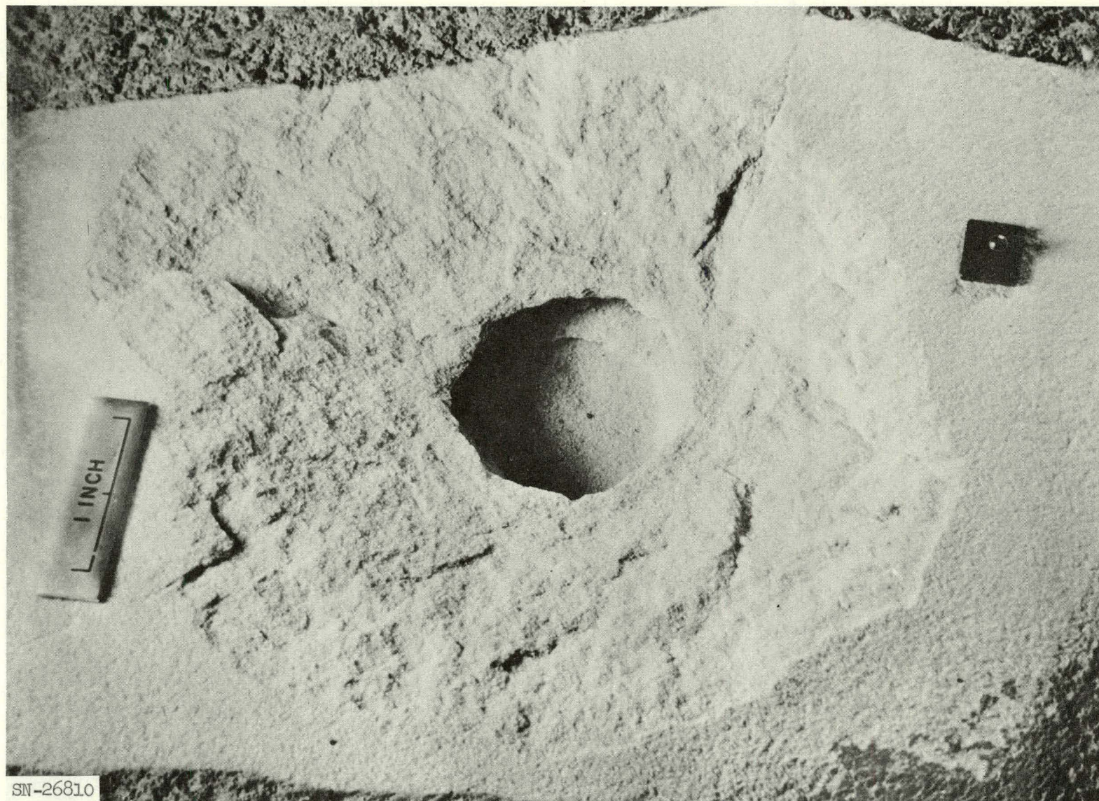
Fig. 2. Slightly oblique photograph of hypervelocity impact crater formed in sandstone by a projectile like that on the black square.
