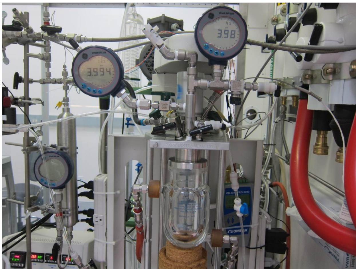
Figure 1: Stirred-cell reactor experimental setup.
