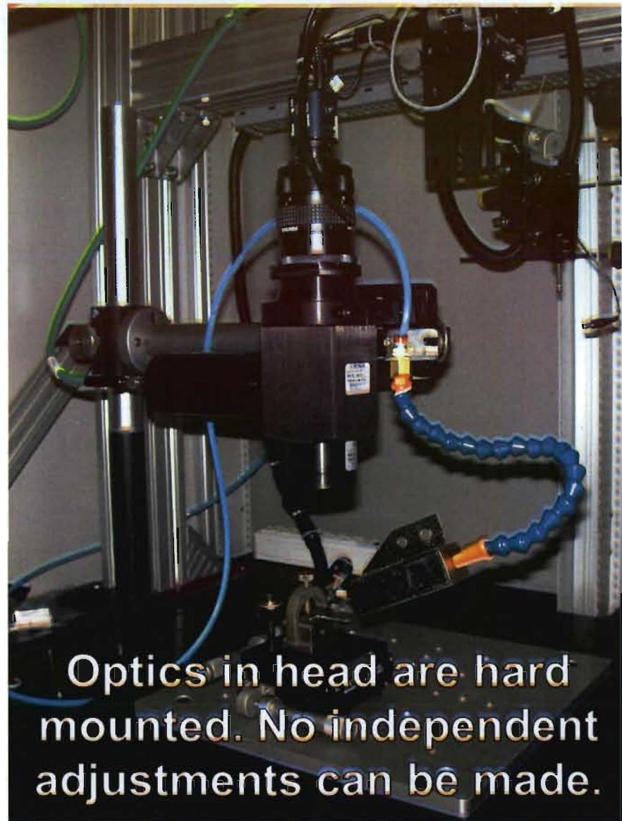
Optics in head are hard mounted. No independent adjustments can be made.
