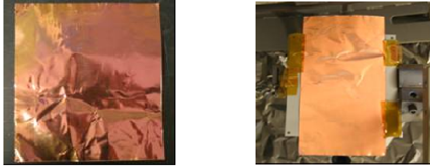
Figure 62. (Left) A 7x7 inch Cu foil with 200 nm \text{CeO}_2 coated on the front and back sides; (Right) \text{TiO}_2 nano-columns grown on a 3x7 inch \text{CeO}_2 coated Cu foil by GLAD.
