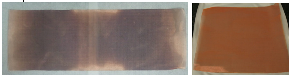
Figure 61. (a) A 3x8 inch Cu mesh coated with 100 nm ZnO film on both sides; (b) A 7x7 inch Cu mesh with 50 nm CeO 2 coated on the front side and 95 nm CeO 2 on the back.
