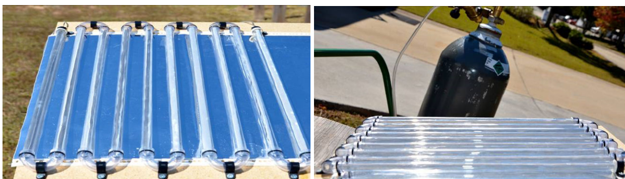
Figure 90. Photos of actual CO 2 reforming reactor prototype built using PN nanostructure on stable stainless steel substrates
