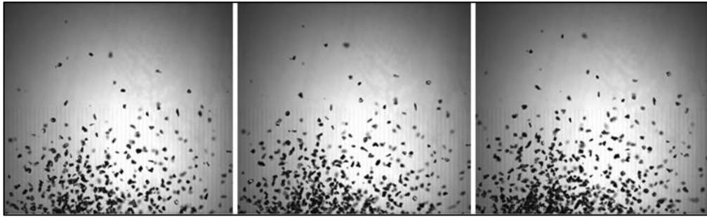
Figure 6: Shadow images for non-spherical particles in dilute section
