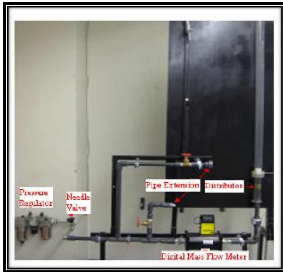
Figure 3.4: Pilot Scale Fluidized Bed
