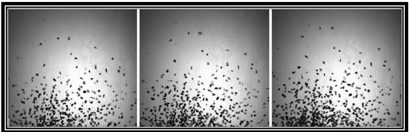
Figure 4.23: Shadow Images of Non-Spherical Particles in Dilute Section
