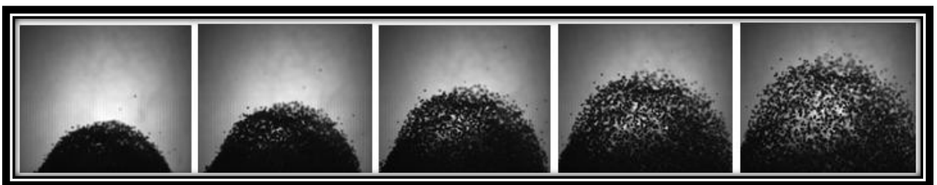
Figure 4.30: Bubble Collapsing for Spherical Particles
