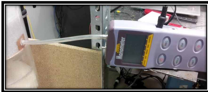
Figure 3.10: Digital Manometer with RS 232 Cable
