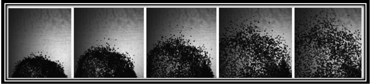
Figure 4.31: Bubble Collapsing for Non-Spherical Particles.
