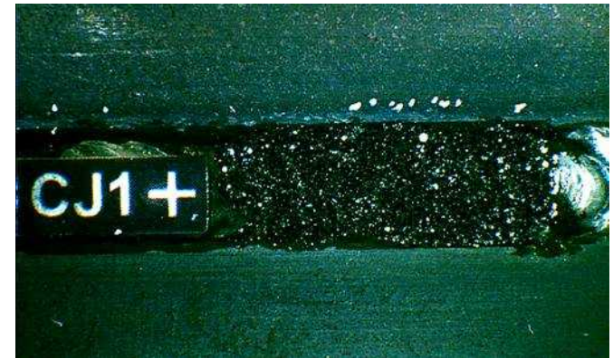
Reflective Particle Tag applied to a weld
