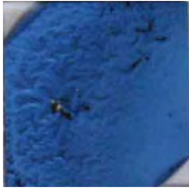
Figure 60: Optical photograph of oxidized NiZr coating after 24 hrs of air annealing at 300°C.
