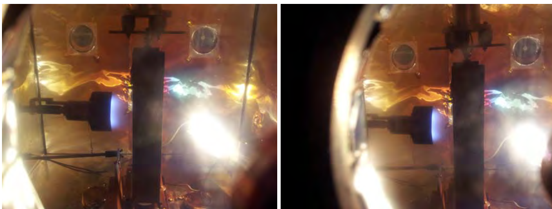
Figure 54: Magnetron sputtering of Cu onto a porous stainless steel tube.
