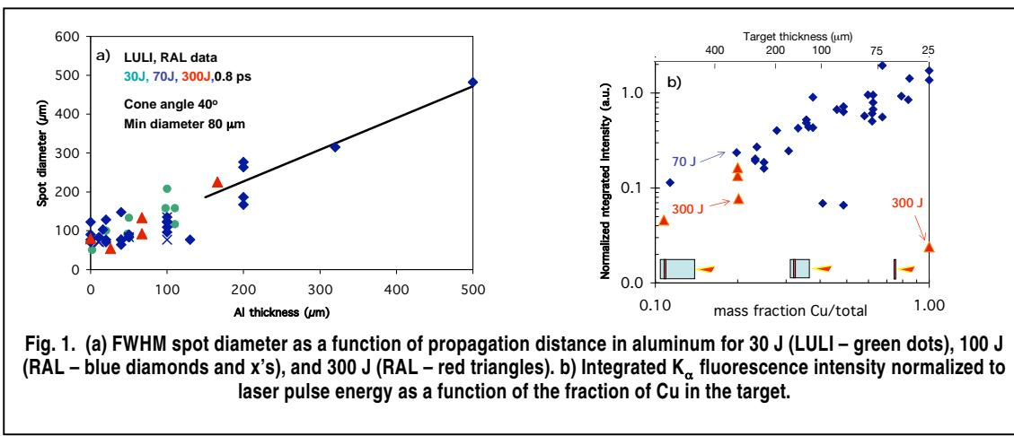
Fig. 1. (a) FWHM spot diameter as a function of propagation distance in aluminum for 30 J (LULI - green dots), 100 J (RAL - blue diamonds and x's), and 300 J (RAL - red triangles). b) Integrated  $K_{\alpha}$  fluorescence intensity normalized to laser pulse energy as a function of the fraction of Cu in the target.
