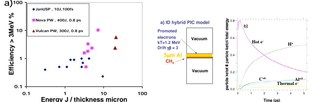
Figure 4: a) Conversion efficiency as a function of foil thickness b) model structure
