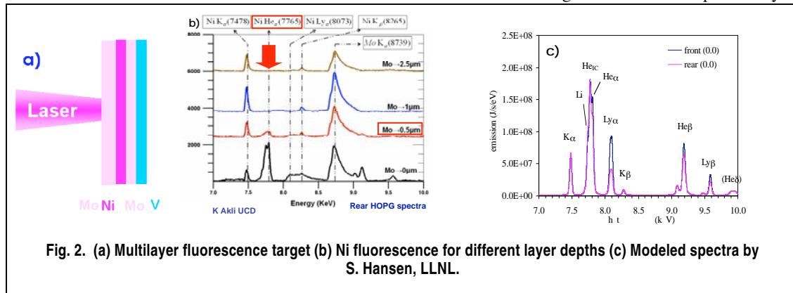
Fig. 2. (a) Multilayer fluorescence target (b) Ni fluorescence for different layer depths (c) Modeled spectra by S. Hansen, LLNL.
