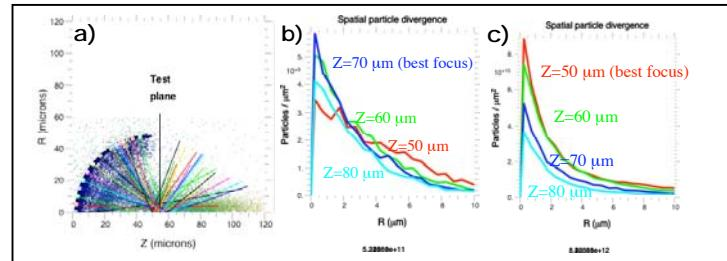
Fig. 3. (a) LSP simulation of 100  $\mu\text{m}$  diameter hemi-shell 3.3 ps after 0.1 ps injection of 1.3 MeV hot electrons showing evolved proton density and typical paths. (b) Transverse proton concentration at various test planes for a 10  $\mu\text{m}$  laser focus. (c) Transverse proton concentration for a 50  $\mu\text{m}$  diameter laser focus.
