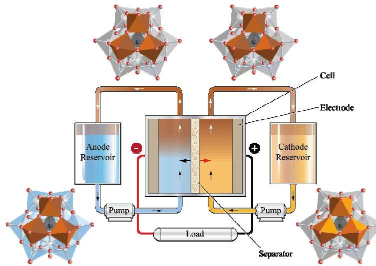
Testing was performed in a cell with serpentine flow field, carbon felt electrodes, and a Nafion 117 membrane.
