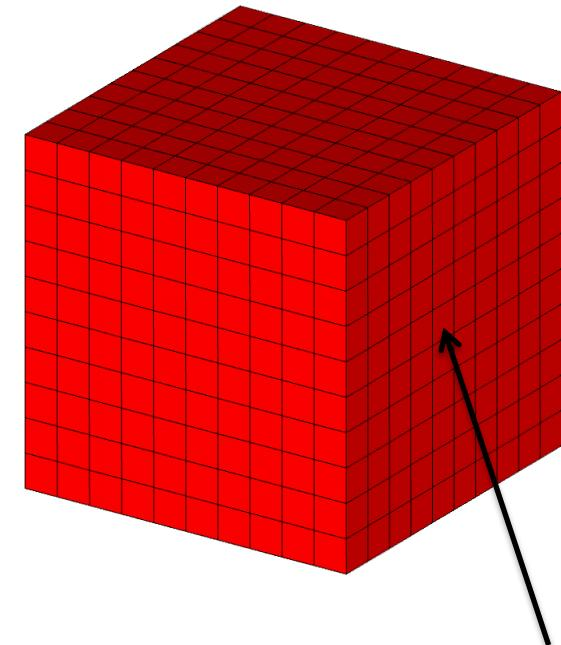
Absorbing BC, Neumann other 5 faces, center point source, solver tolerance =  $10^{-8}$
