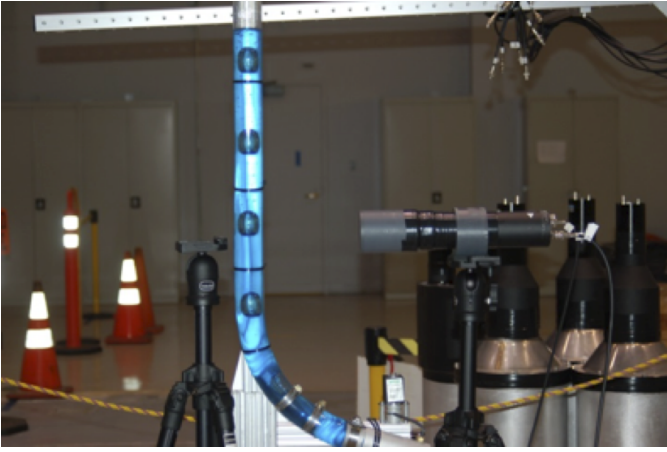
Fig. 8. Experimental setup of the bubble acquisition system: a PMT is placed opposite of a source stand with the glycerol tube and bubbles placed in between
