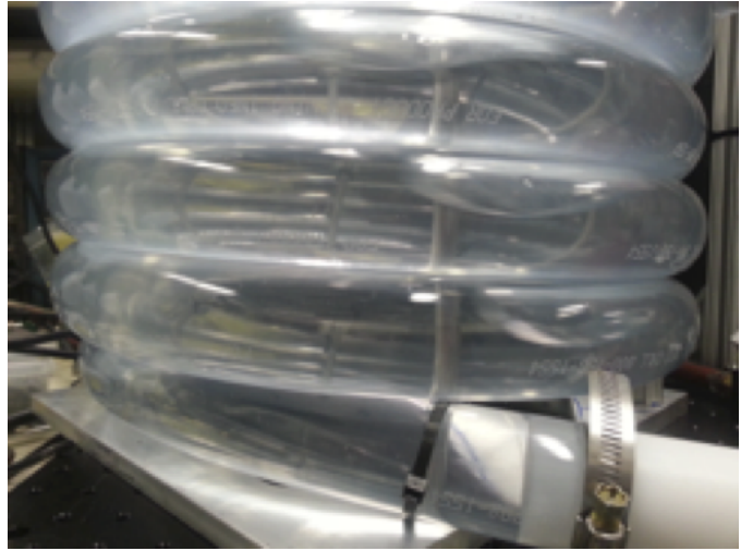
Fig. 5. Helical mask with mineral oil and air injected.
