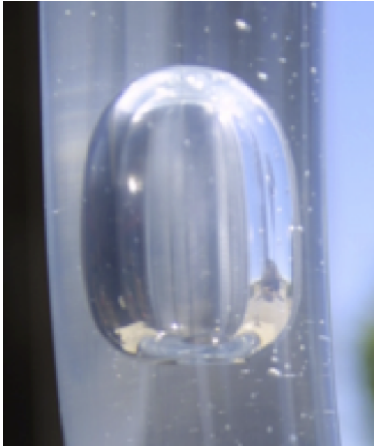
Fig. 4. A bubble transiting up the tube filled with glycerine.
