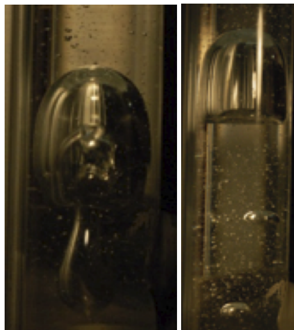
Fig. 3. First image shows bubble as it emerges from the solenoid valve. Second image shows small after bubbles following the main bubble up the tube.
