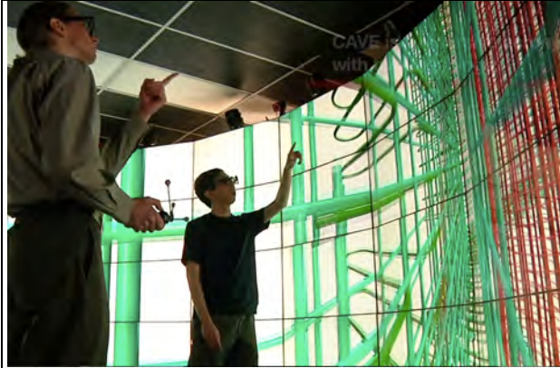
CAVE2 displays a 3D model of a section of the rebar cage of the San Francisco-Oakland Bay Bridge created by American Bridge Company/Fluor Enterprises. A UCSD Structural Engineering student and UCSD computer science professor Jurgen Schulze ported to virtual reality. It is displayed with Calit2's CalVR software.
