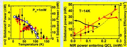
• SB’s disappear at  $T \sim 120\text{K}$ , [like in THz QCL’s] and the conversion efficiency is  $\propto$  (ISBT polariton density)
