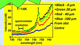
• SB’s appear only when the laser spot hits slot opening and when Ti:saphire photon energy is high enough to create ISBT polaritons by interband excitation.
