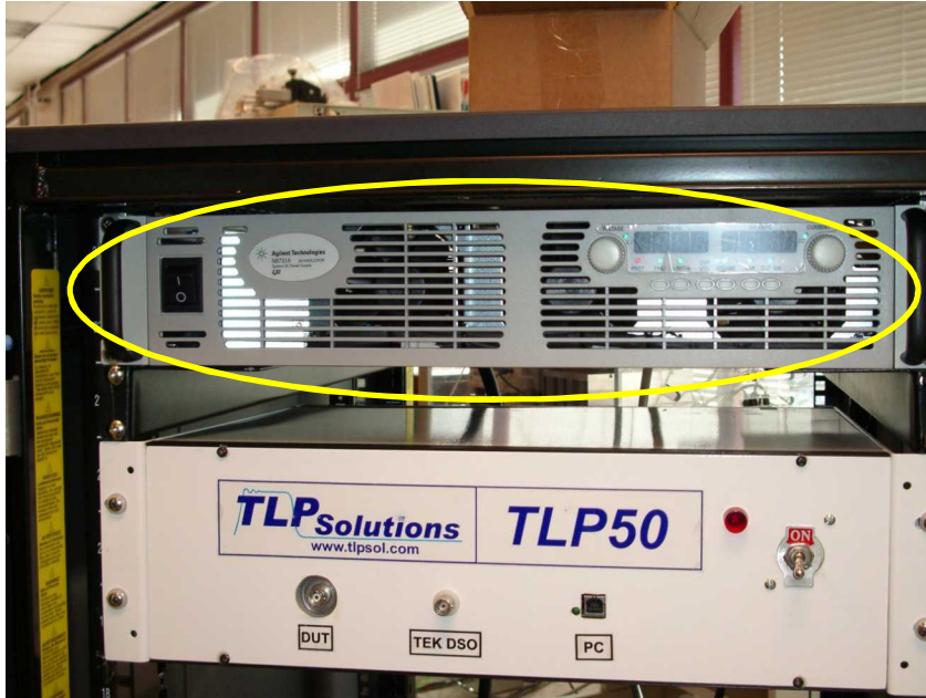
3200 W power supply (400 A, 8 V)
