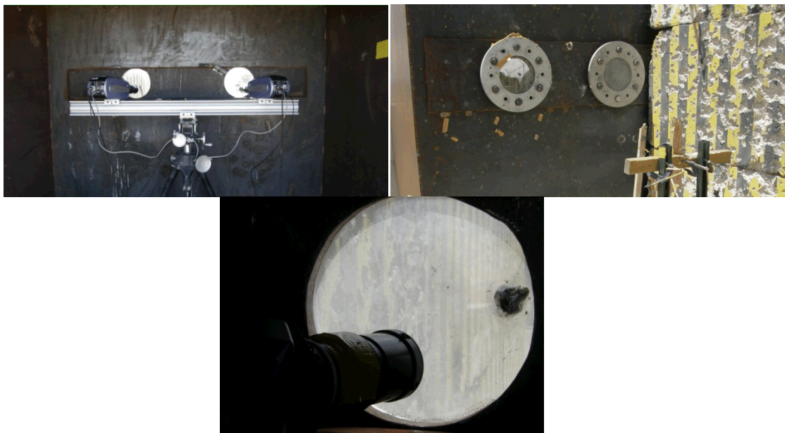
Fig. 3. Shimadzu cameras in the protective enclosure. Thick lexan sheets cause large distortions. Bottom image shows a fragment lodged in the lexan after the test.
