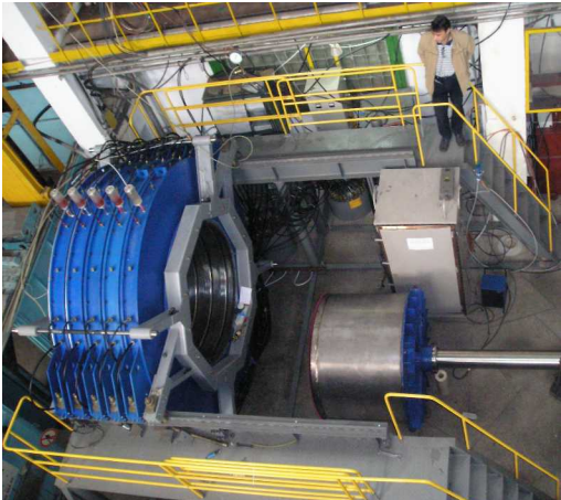
Fig. 30. 5, 1-MA LTD cavity voltage adder with the cylindrical cathode stock and visible outside of the cavities
