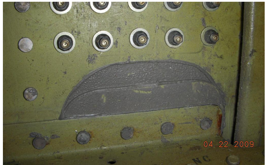
(A) Zero Edge distance, (B) Tooling mark
