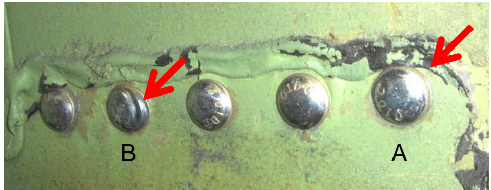
(A) Zero Edge distance, (B) Tooling mark
