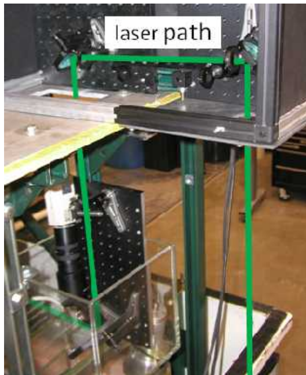
Figure 15. The optical path maintains approximate alignment as the tank lid is raised or lowered.
