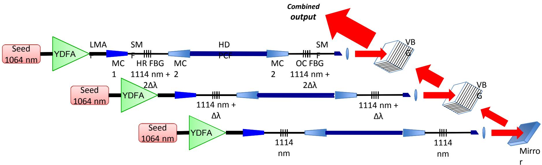
*Several broadband COTS kW-class lasers can be spectrally compressed at different wavelengths via proper selection of fiber Bragg gratings and combined using SBC*
