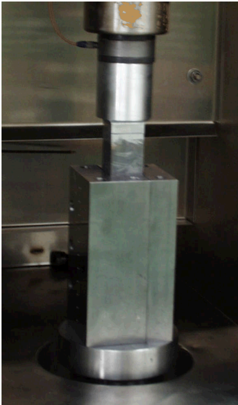
Thick wall for rigid confinement.
