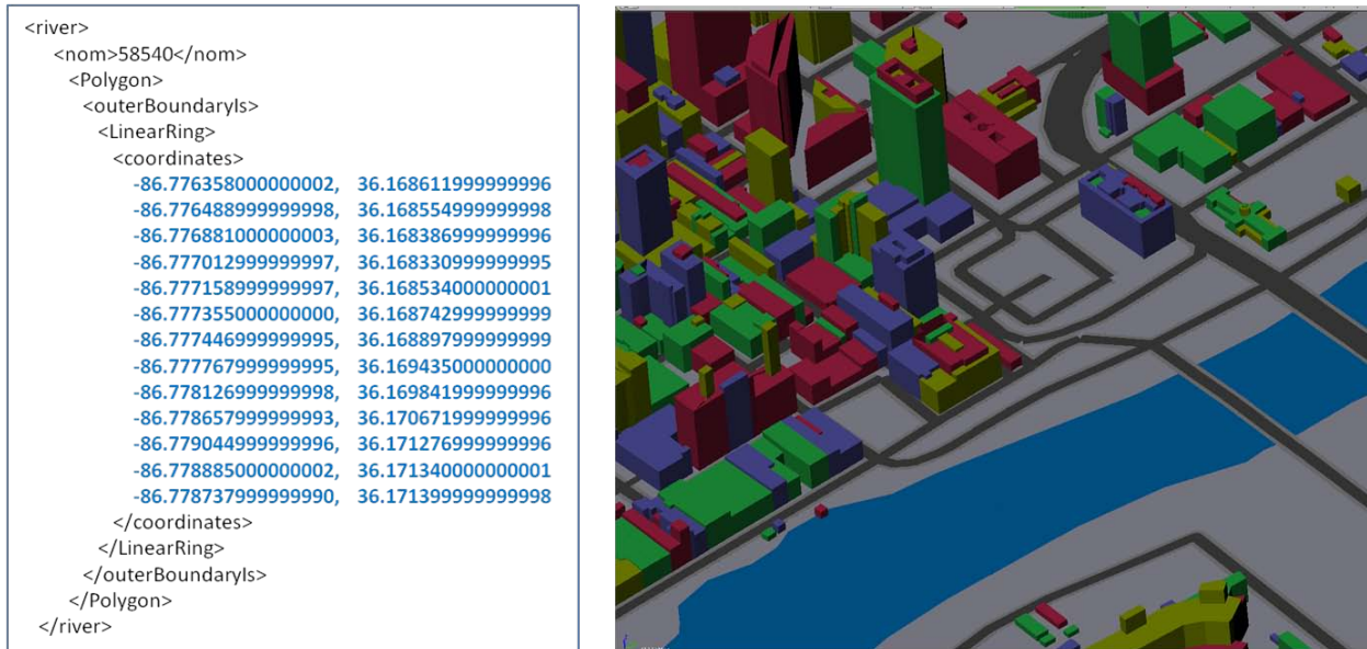
Figure 4: XML description of a section of river, and an illustration of the model including streets, sidewalks and river
