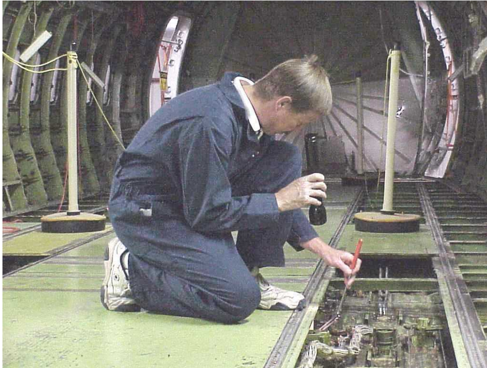
Detailed visual inspection of 737 floor beams using a flashlight and mirror.
