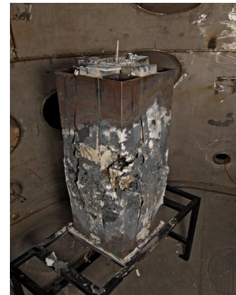
Fuel bundle assembly after the test.
