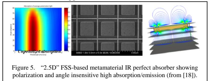
Figure 5. “2.5D” FSS-based metamaterial IR perfect absorber showing polarization and angle insensitive high absorption/emission (from [18]).
