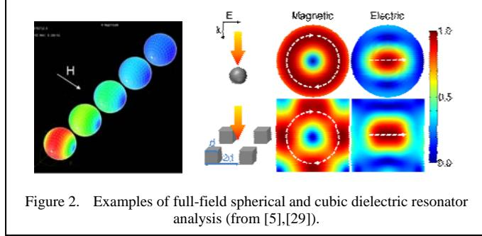
Figure 2. Examples of full-field spherical and cubic dielectric resonator analysis (from [5],[29]).
