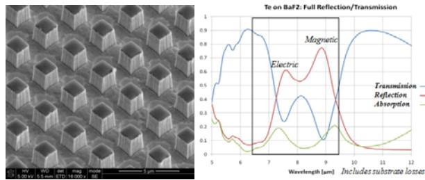
Figure 7. Te dielectric resonator optical metamaterial showing distinct electric and magnetic resonances in the LWIR (from [29]).
