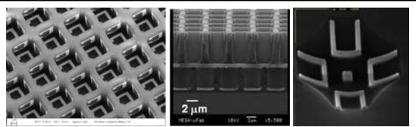
Figure 4. Single- and multilayer Membrane Projection Lithography-based (MPL) resonator and non-resonant (artificial dielectric) materials, Self-Aligned MPL-based tilted antennae absorbers/emitters.
