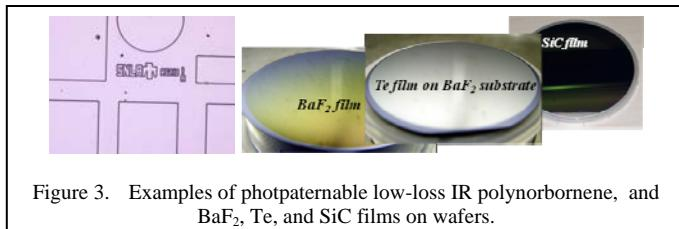
Figure 3. Examples of photopatternable low-loss IR polynorbornene, and BaF<sub>2</sub>, Te, and SiC films on wafers.
