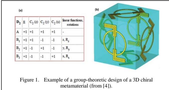
Figure 1. Example of a group-theoretic design of a 3D chiral metamaterial (from [4]).
