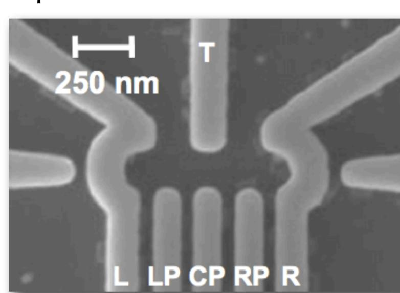
In double quantum dots, electrons circulate from source to dot 1 to dot 2 to drain.
