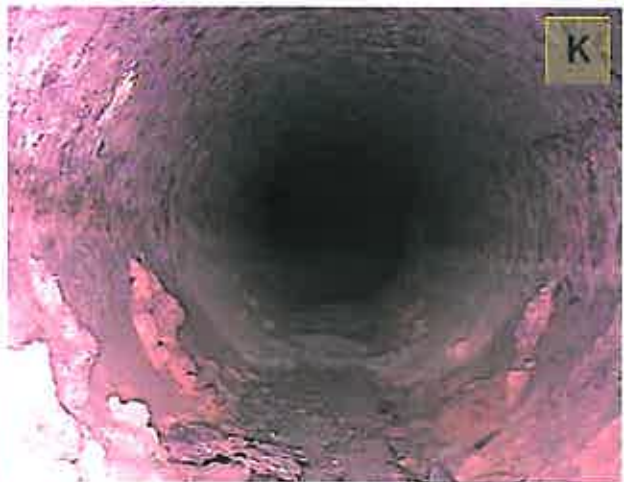
Figure 3-13. View of Region Downstream of Third Elbow (a distinct color change, perhaps a transition to a completely dry region)
