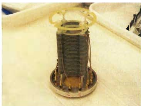
Fully assembled ^{235}\text{U} counter with a total mass of 113 mg
