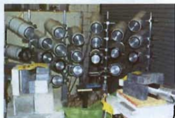
FIG. 3. (Color online) The FIGARO array, consisting of 20 EJ301 neutron detectors and a \text{BaF}_2 \gamma -ray detector.
