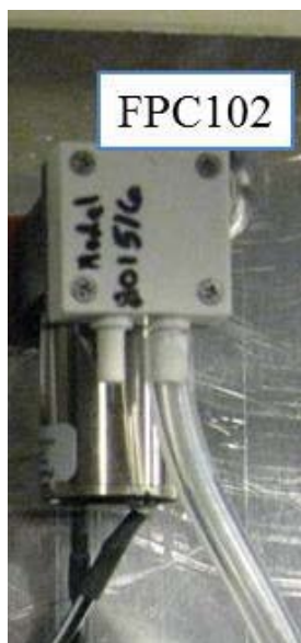
Figure 23. FPC101 and FPC102 pumps (Sensidyne Inc. Model 810516).
