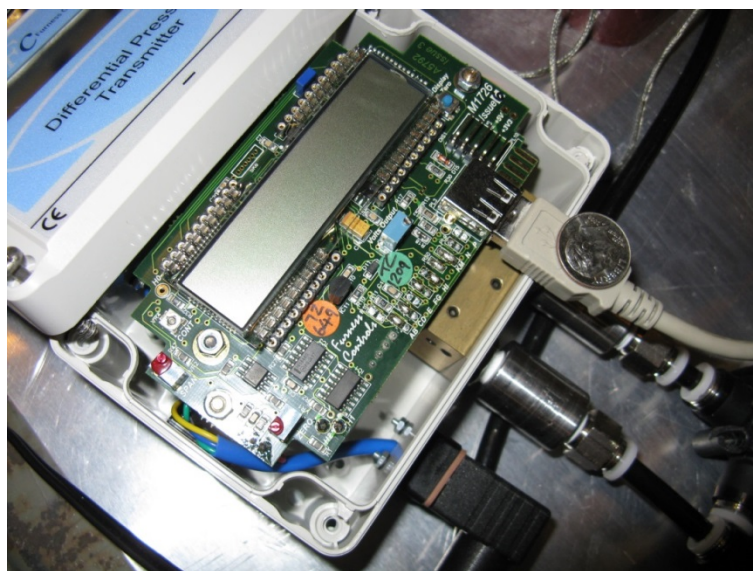
Figure 30. PI 101 pressure gauge measures the tested filter (inches of water column, in WC). Furness Inc model #FCO332 has integrated pressure transducer and panel display.
