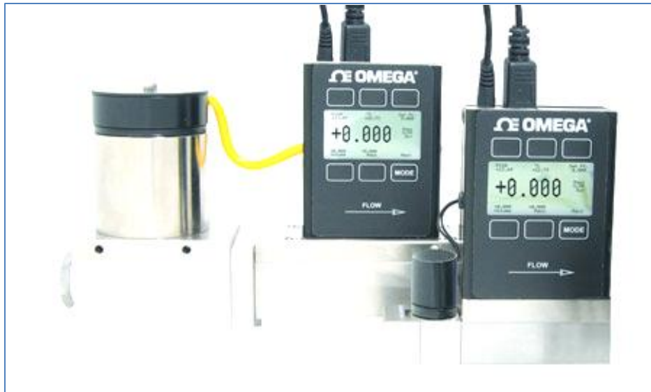
Figure 22. FIC101 and FIC102 flow controllers.
