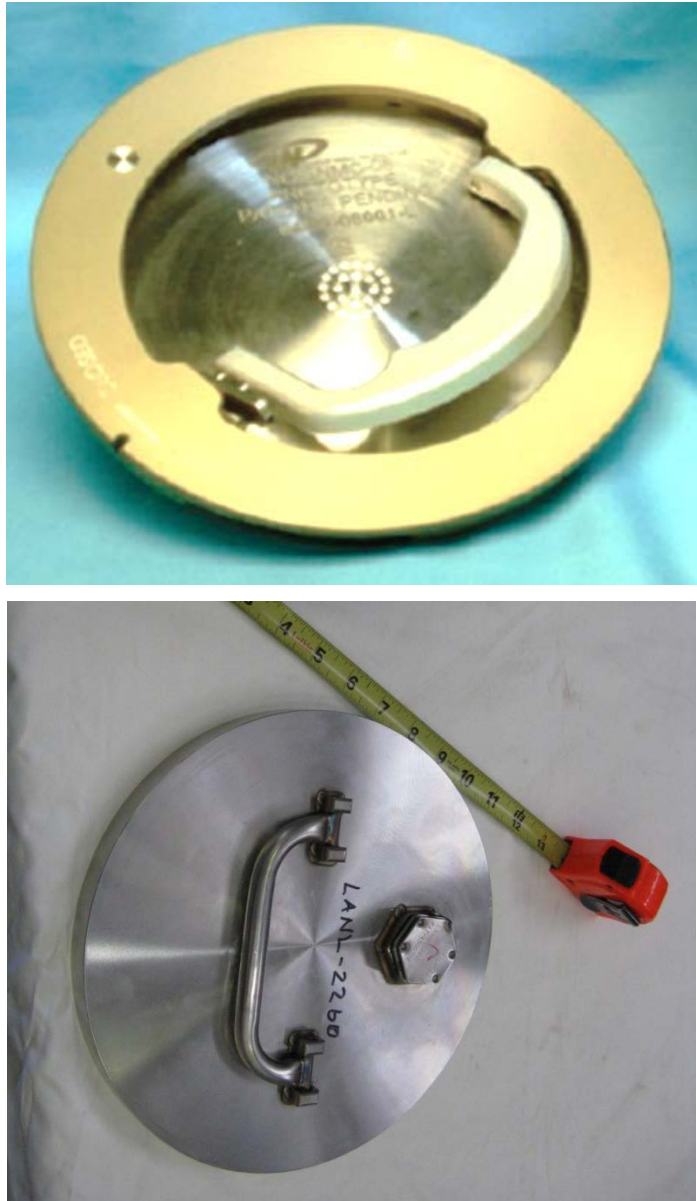
Figure 25. N202 The filter to be tested is integrated into the lid of a SAVY or Hagan canister.
