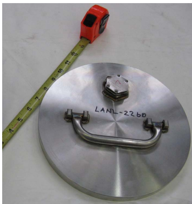
Figure 3. Hagan type canister lid with hexagonal filter port.
