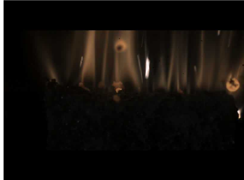
Video of a propellant burning at 100 psi in nitrogen (Ward, Atwood, and Bui, 2006).
