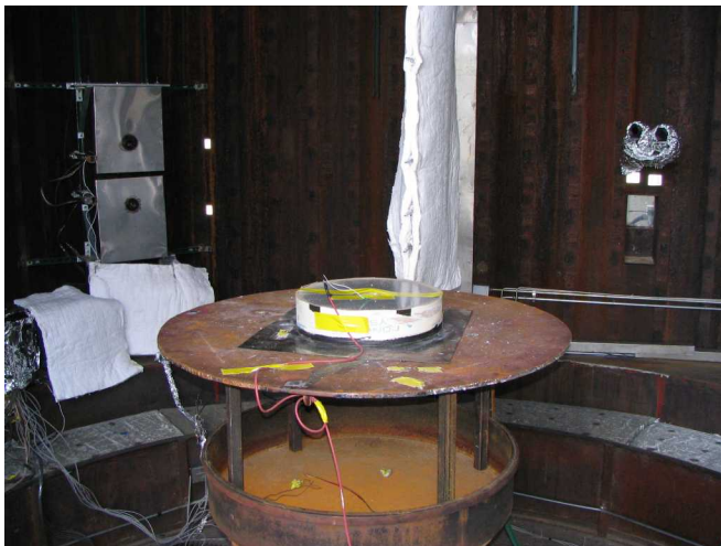
Upward-facing propellant charge pre-test
