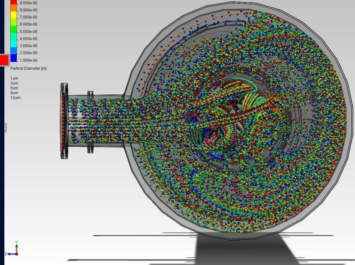
Inlet view presents a well-mixed aerosol upon entrance into the measurement tube.
