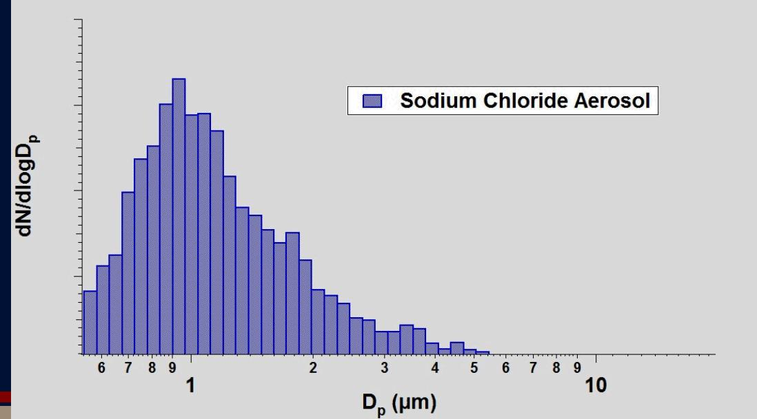
Observed large fraction of small particles (<1  $\mu\text{m}$ )
